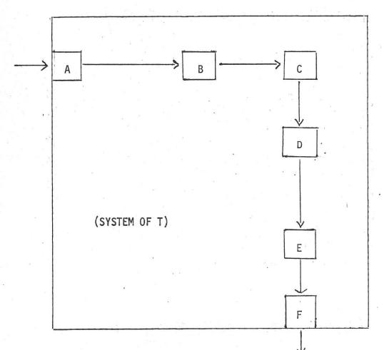
This system T consists of six components in series (A,B,C,D,E,F). PROBLEM: Predict the system reliability for a target of 1000 hours.
